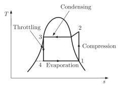
T-s diagram for given Refrigeration cycle is given above
